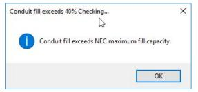
This also can be run on existing conduit runs that have either wirefill or panels and circuits assigned. Select the conduit run, and in the tool menu select "Check for exceeding fill %.
