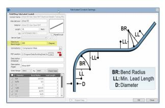
This can also be run on existing conduit runs by selecting the run and in the tool menu select "Check for Exceeding Max Angle".
